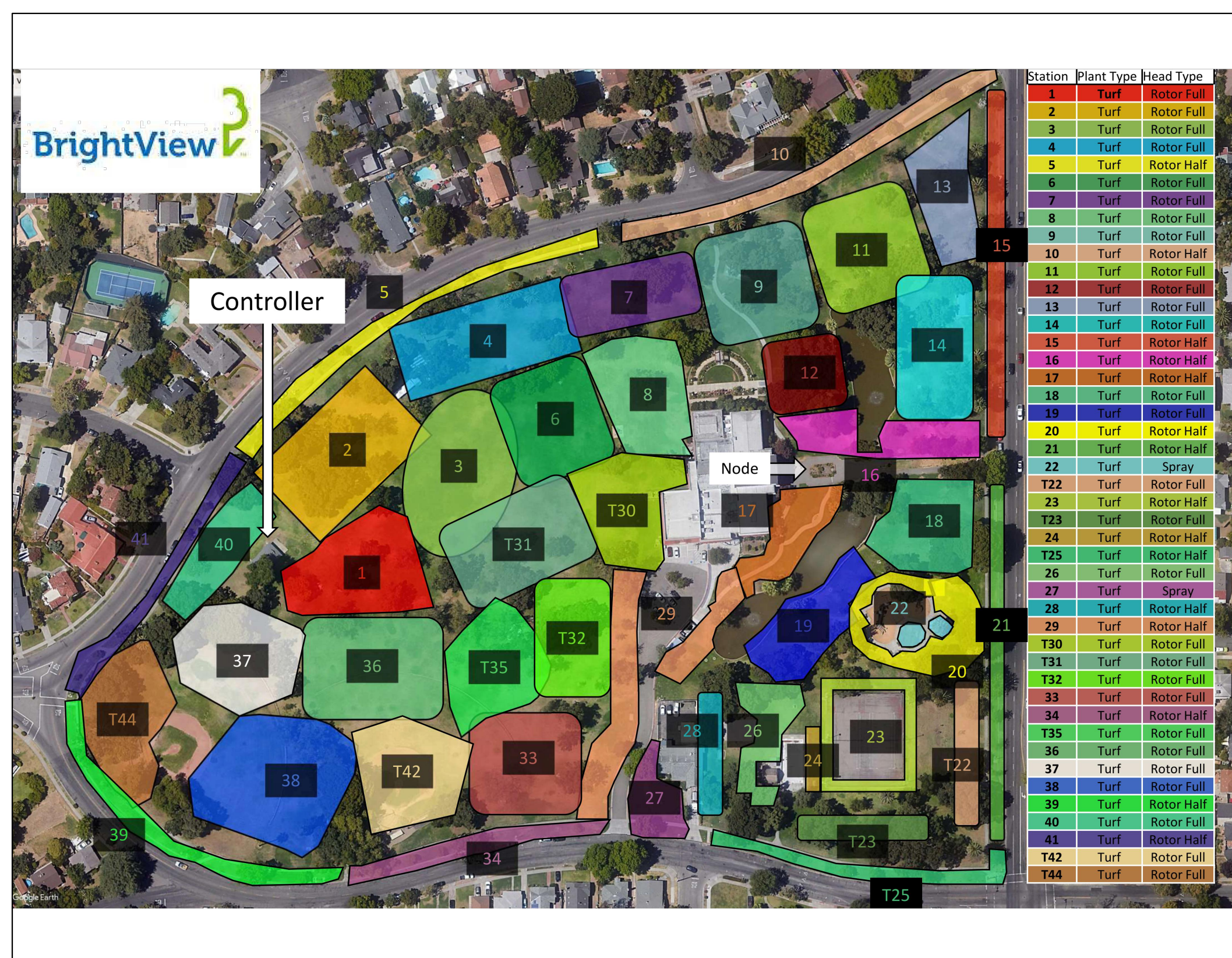
EXISTING CIRCUITS VICTORY PARK SITE NO SCALE
